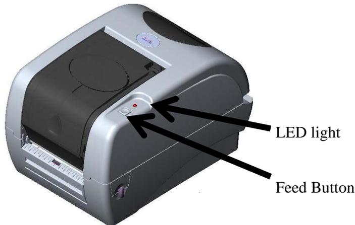
**Label Index Procedures:** Only use these steps if the printer prints a label then stops and the LED turns Flashes RED
